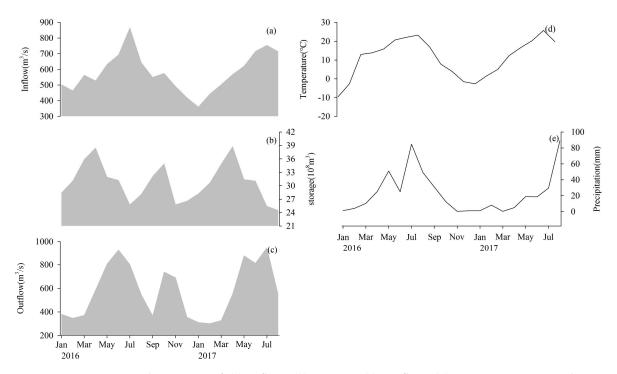
**Figure 3.** Seasonal variation of (**a**) inflow, (**b**) storage, (**c**) outflow, (**d**) air temperature, and (**e**) precipitation amount from January 2016 to August 2017.
