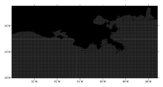
**Figure S2.** Mesh of the nGoM domain (longitude: 94°W–87.6°W; latitude: 27.9°N–30.7°N; horizontal resolution: 1 km; number of vertical layers: 24).
