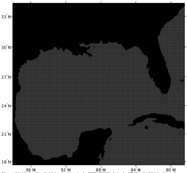
96 W 92 W 88 W 84 W 80 W **Figure S1.** Mesh of the GoM domain (longitude: 98°W–79°W; latitude: 17.6°N–34.3°N; horizontal resolution: 5 km; number of vertical layers: 36).
