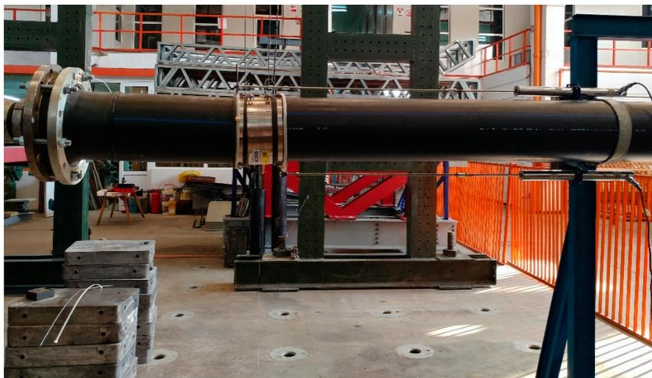
**Figure 3.** System consisting of two pipeline sections joined by a Flexseal SC200.
