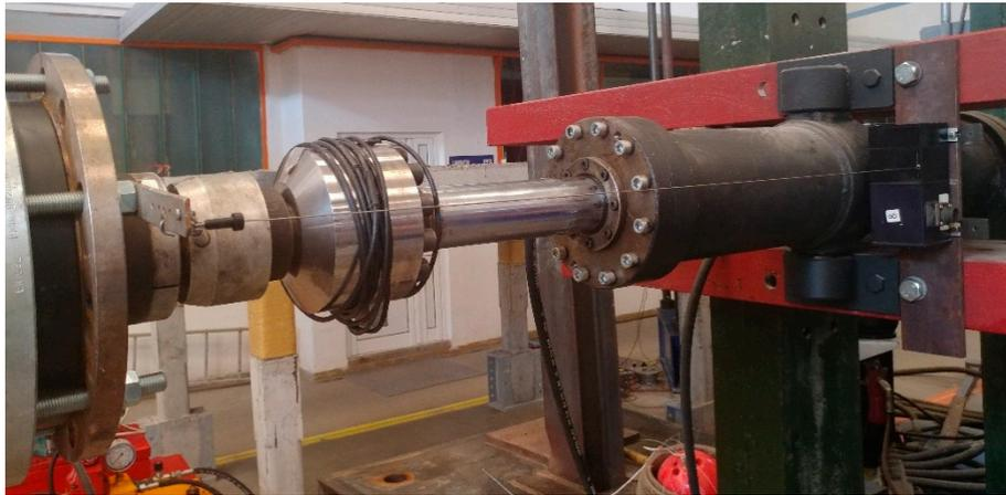
**Figure 4.** AEP 100 kN Force Cell and Celesco PT5AV wire displacement transducer.
