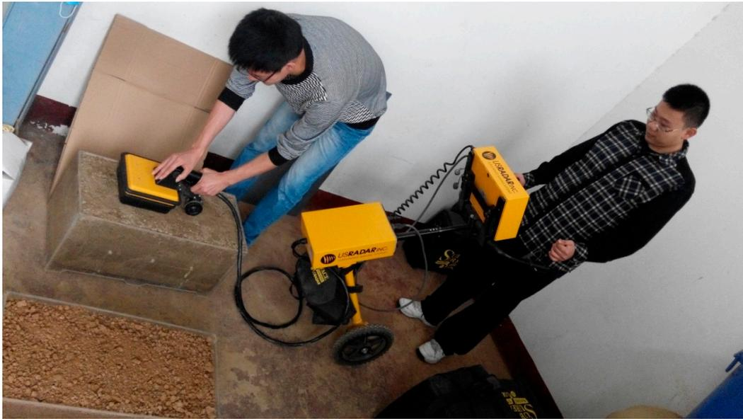
Figure 4. GPR measurement in the laboratory box.
