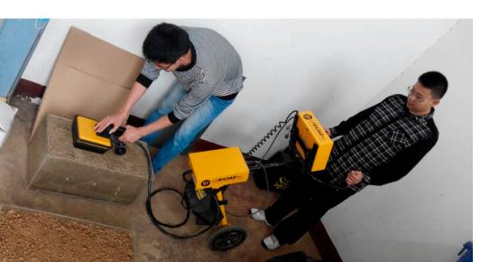
Figure 4. GPR measurement in the laboratory box.
