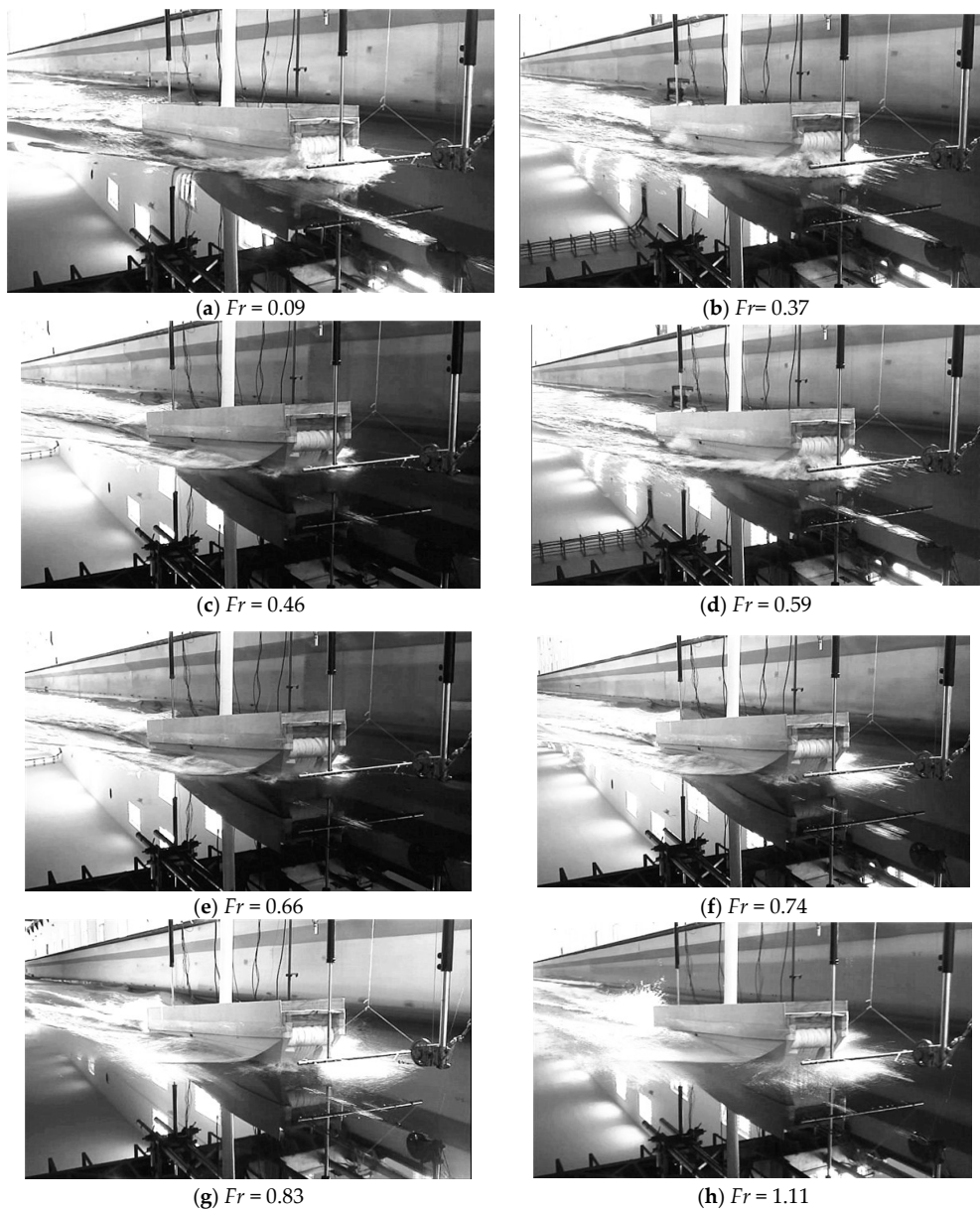
Figure 13. Snapshots of the planing trimaran at different speeds. \Delta = 145\text{ kg} , Q = 150\text{ m}^3/\text{h} .
