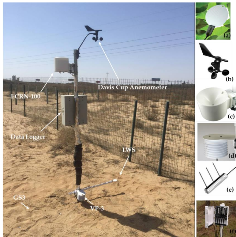
Figure 3. Experimental setup. Instruments include: (a) LWS; (b) Davis Cup Anemometer; (c) Rain gauge (ECRN-100); (d) Air relative humidity and temperature sensor (VP-3); (e) Soil temperature and moisture sensor (GS3); (f) Data logger (EM50) inside the security box.
