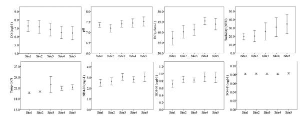
**Figure 3.** Physical-chemical parameters (mean  $\pm$ SE), dissolved oxygen (DO), pH, electrical conductivity (EC), turbidity, temperature, ammonium-N, nitrate-N, and phosphate-P of water quality measured at different sampling sites in Kilombero Valley, where Site 1 and 2 are upstream sites, Site 3- middle site, and Sites 4 and 5 are downstream sites.
