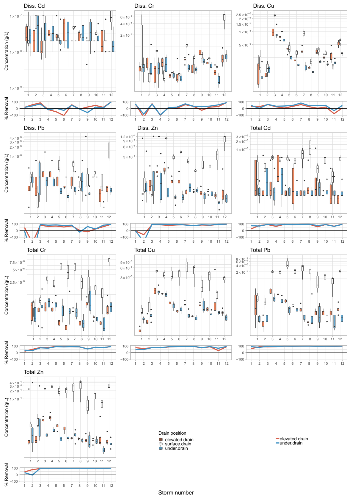
Figure 5. Removal efficiencies for total and dissolved heavy metals at elevated drain and under drain positions. Removal efficiencies below -100\% (or over 100\% export) are not shown, and why some line graphs appear broken.
