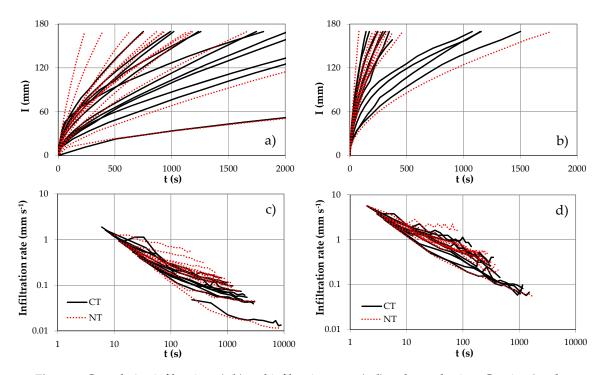
**Figure 2.** Cumulative infiltrations (a,b) and infiltration rates (c,d) at the study sites, Gravina (on the left) and Candela (on the right), under conventional tillage (CT) and no-tillage (NT). Note that I(t) relationship of Gravina was truncated at t = 2000 s; lost information can be assumed from Table 4.
