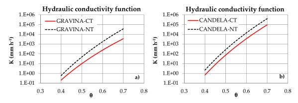
**Figure 6.** Hydraulic conductivity functions obtained with BEST-steady at Gravina (**a**) and Candela (**b**) sites.
