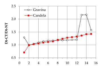
**Figure 3.** Ratio between the mean infiltration time for water infiltration in CT and NT during the Beerkan runs against the number of the applied volumes of water.
