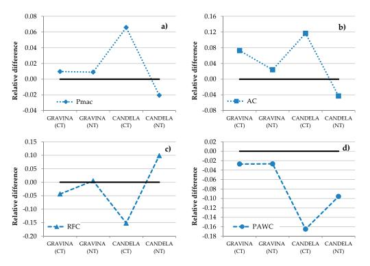
**Figure 9.** Relative differences between measured mean values and optimal mean values for macroporosity (**a**), air capacity (**b**), relative field capacity (**c**) and plant available water capacity (**d**), according to the Table 1.
