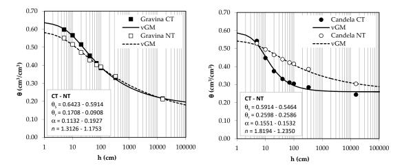
**Figure 7.** Measured (points) and modelled (lines) soil water retention data (van Genuchten model, vGM) for conventional tillage (CT) and no-tillage (NT) of Gravina (on the left) and Candela (on the right) sites. Parameters of vGM ( $\theta_s$ ,  $\theta_r$ ,  $\alpha$ , and n) are also reported ( $\alpha = 1/\text{cm}$ ).
