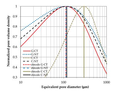
**Figure 8.** Normalized pore volume distributions and the corresponding modal diameters (d<sub>mod</sub>) of the four site–soil management combinations (G, Gravina; C, Candela; CT, conventional tillage; NT, no-tillage), calculated according to Reynolds et al. [62].
