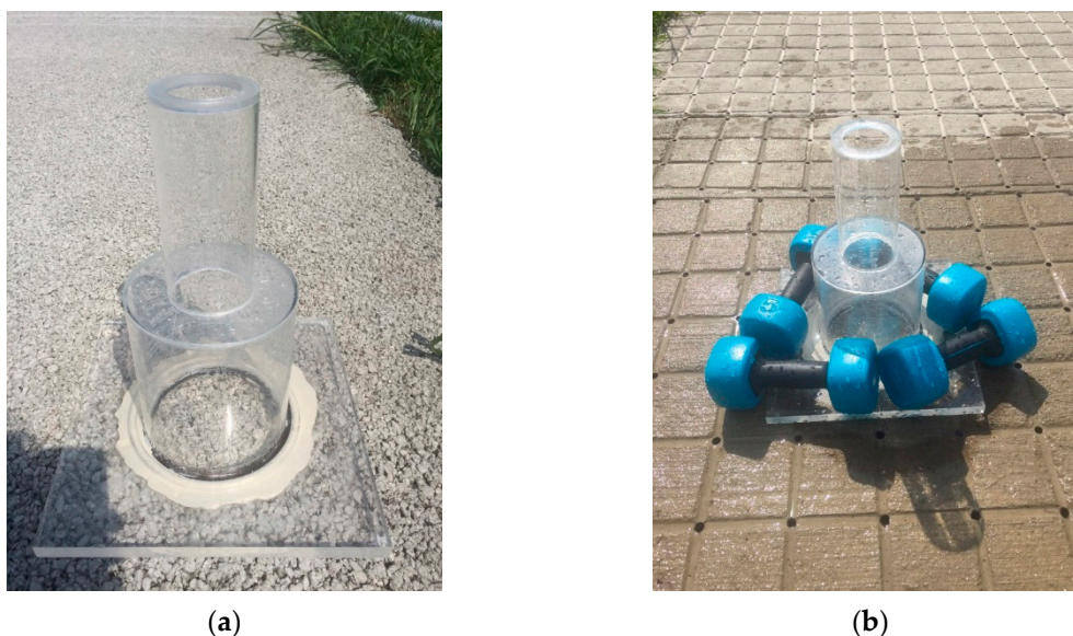
Figure 6. (a) The structure of the NCAT permeameter used in this study. (b) Usually, some weights were placed on the base to stabilize the instrument and to help secure the seal between the instrument and the test pavement.
