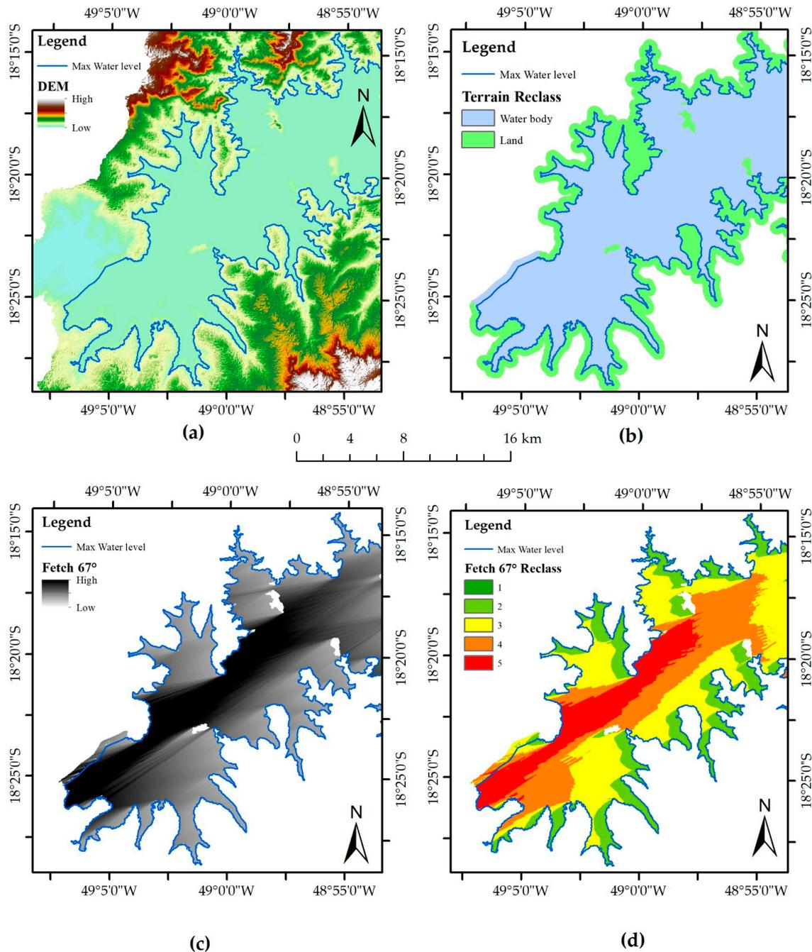
**Figure 6.** (a) Digital Elevation Model, (b) reclassified Land/Water raster, (c) fetch of 67.5° wind direction, and (d) reclassified raster of the fetch of 67.5°.
