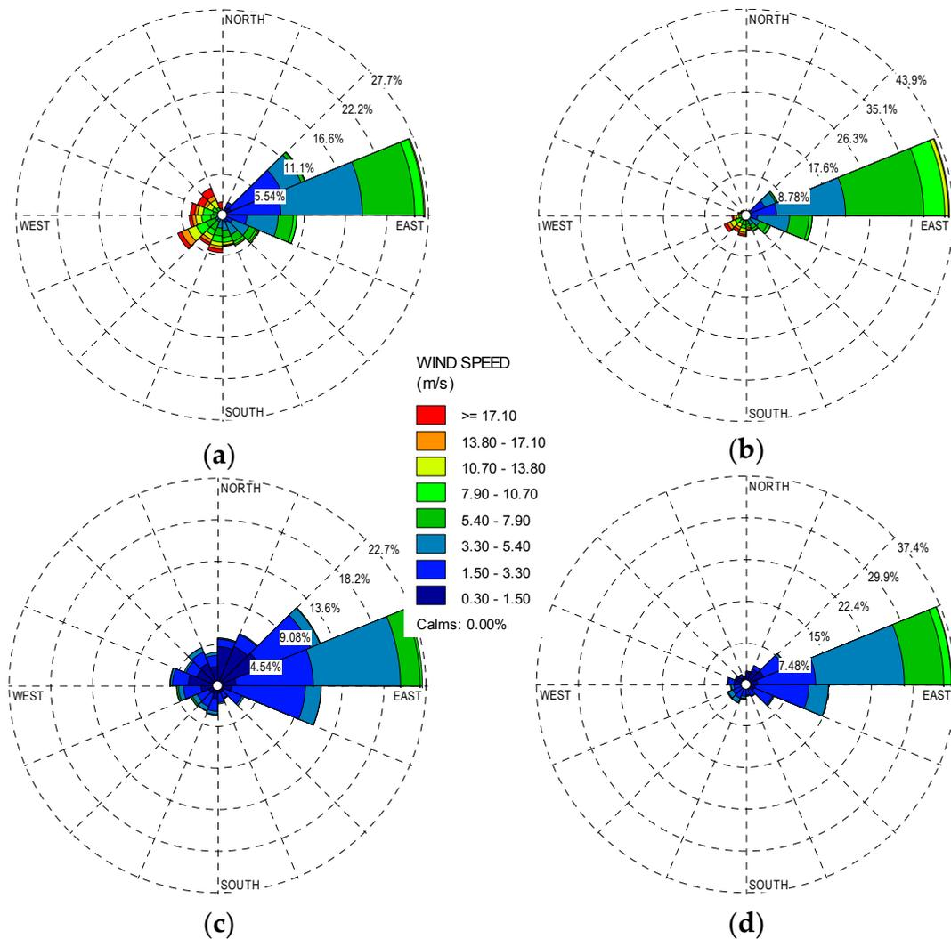
**Figure 4.** The wind rose plots, separated by rainy (a) and dry (b) seasons of SODAR, and rainy (c) and dry (d) seasons for the weather station.
