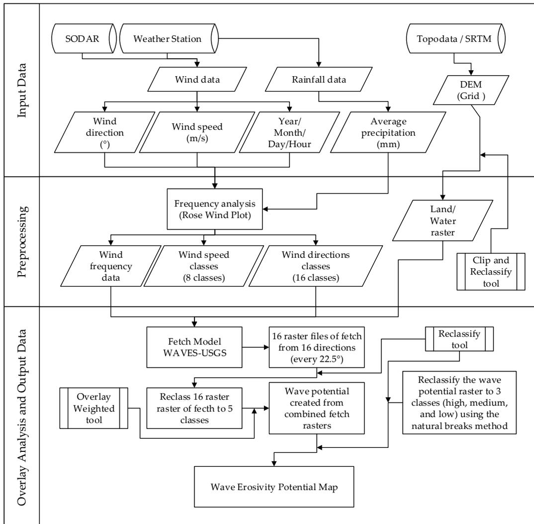
Figure 2. Shoreline Wave Erosivity Potential flowchart.
