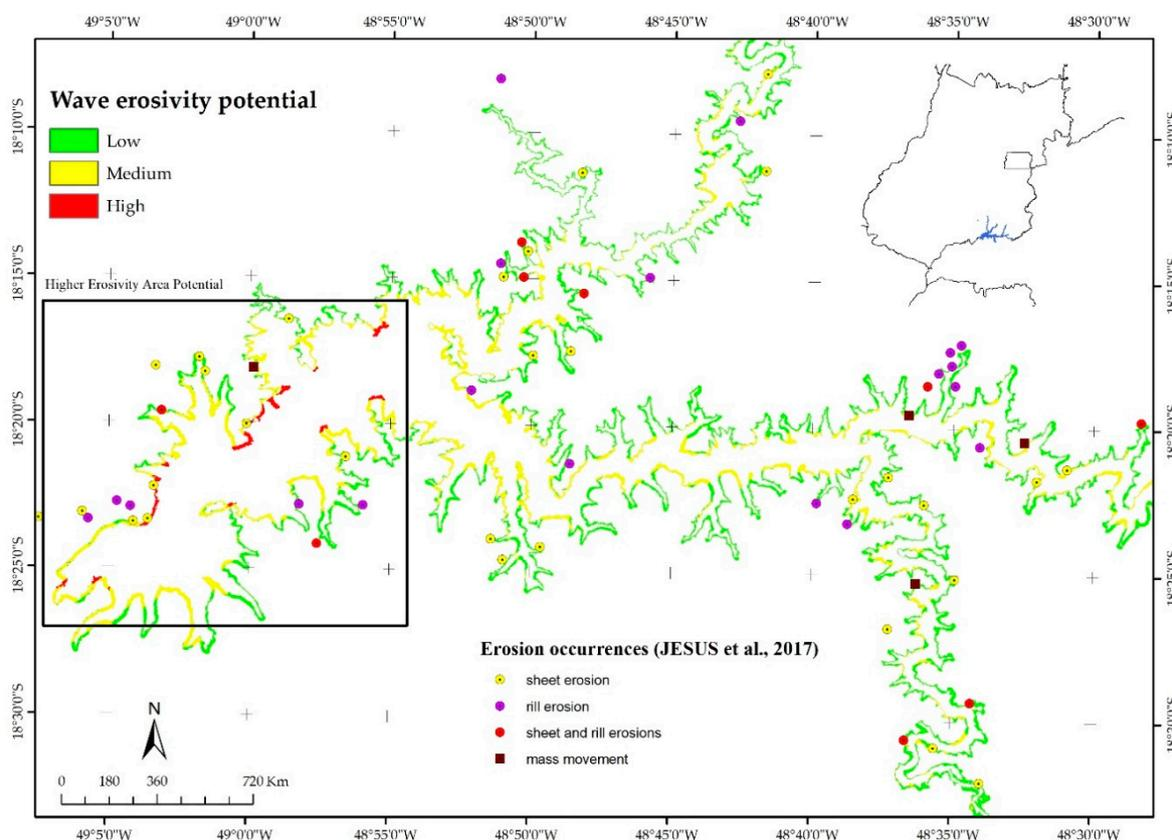
Figure 7. Wave erosivity potential map of the Itumbiara Dam reservoir.
