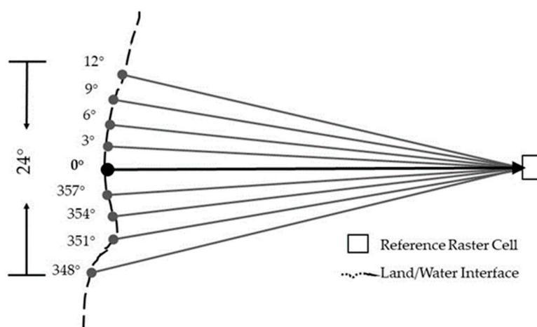
Figure 3. Schematic SPM method to evaluate the wind fetch model.
