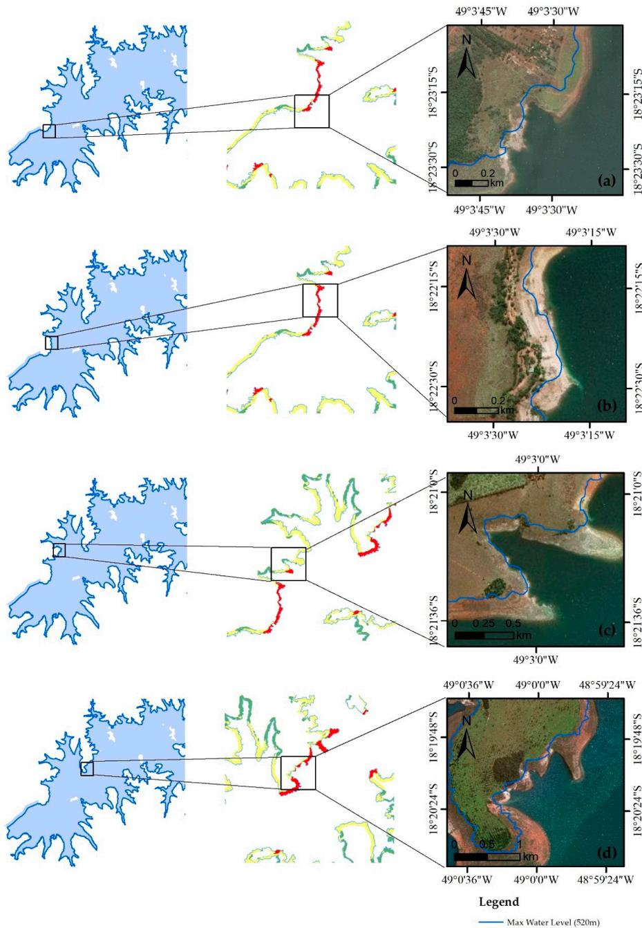
**Figure 10.** Satellite imagery of the shoreline of erosion sites that have a direct relationship with high values of wave erosivity potential. (a) Area 1. (b) Area 2. (c) Area 3. (d) Area 4.
