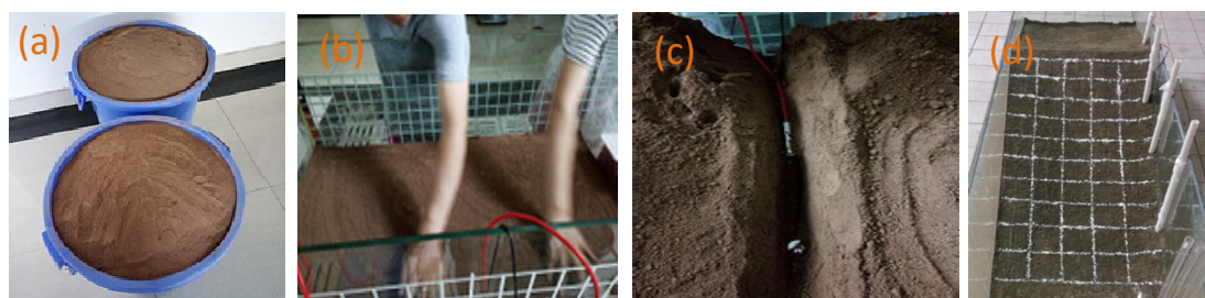
Figure 5. The procedures of tailings dam construction. (a) Tailings sample; (b) tailings dam construction; (c) tailings dam construction; (d) displacement monitor.
