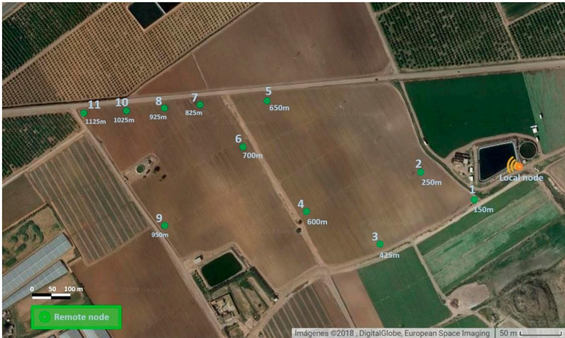
**Figure 11.** Aerial view of the location of the local control node and the remote capture nodes (source: DigitalGlobe, European Space Imaging).
