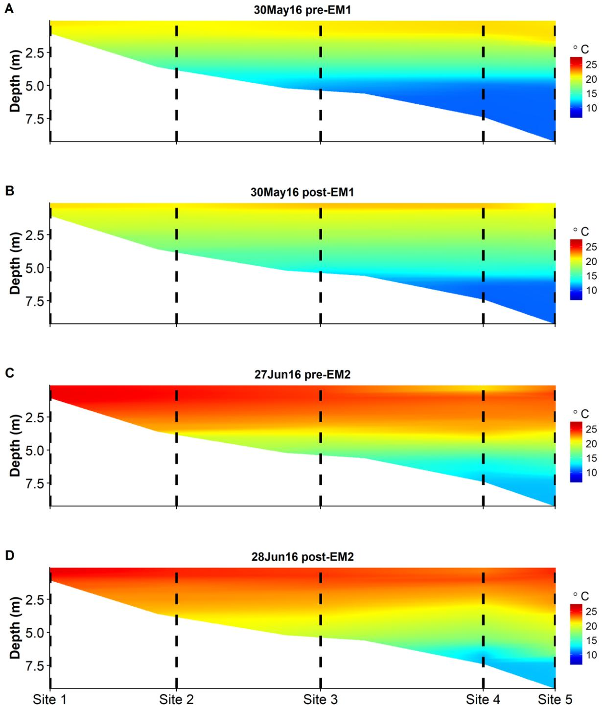
**Figure S.1:** Temperature across a longitudinal cross-section in Falling Creek Reservoir (FCR) from immediately before EM1 (A, 30 May 2016), immediately after EM1 (B, 30 May 2016), immediately before EM2 (C, 27 June 2016) and immediately after EM2 (D, 28 June 2016). Contours are interpolated from CTD casts taken at the upstream and deepest sites (denoted by the vertical lines; upstream sampling sites are shown on the inset in Fig. 1).
