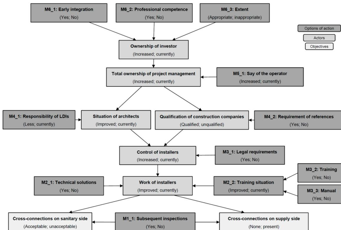
**Figure 3.** Bayesian belief network of actors, measures, and targets regarding cross-connections in semi-centralized water infrastructures.
