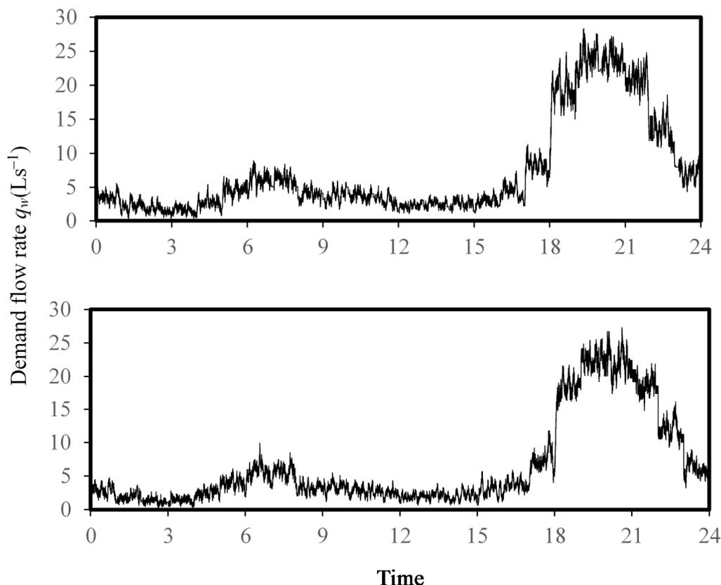
**Figure 5.** Total demand flow rates: (a) maximum daily consumption ( $590.0 \text{ m}^3 \cdot \text{d}^{-1}$ ); (b) minimum daily consumption ( $534.8 \text{ m}^3 \cdot \text{d}^{-1}$ ).
