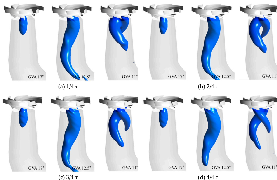
Figure 17. Iso-surface distributions of vortex rope with GVAs of 17° (left), 12.5° (middle), and 11° (right) during one runner revolution: (a) 1/4 \tau , (b) 2/4 \tau , (c) 3/4 \tau , and (d) 4/4 \tau in the draft tube.
