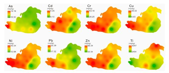
**Figure 2.** Spatial distribution patterns of As, Cd, Cr, Cu, Ni, Pb, Zn, and Ti in surface sediments from Lake Dali.
