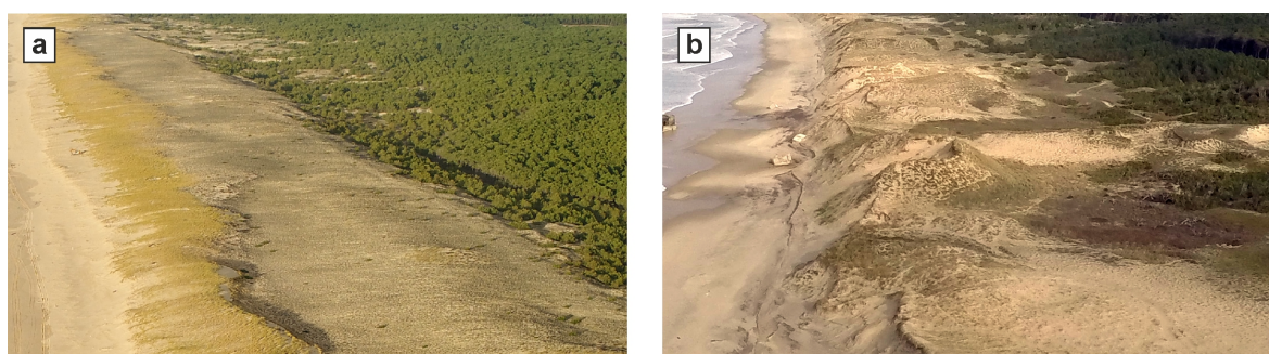
Figure 1. Aerial photographs in Southwest France of (a) a reprofiled coastal dune designed as an alongshore-uniform feature with limited natural community diversity at Truc Vert, contrasted with (b) an alongshore-variable dune field with more natural community diversity at Anse du Gulp, Southwest France (Ph. V. Marieu).
