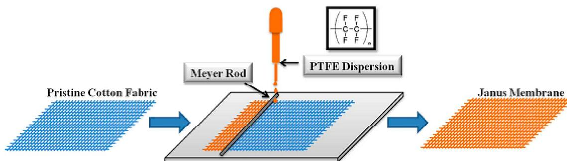
Figure 7. Schematic of the fabrication of Janus membrane [39].
