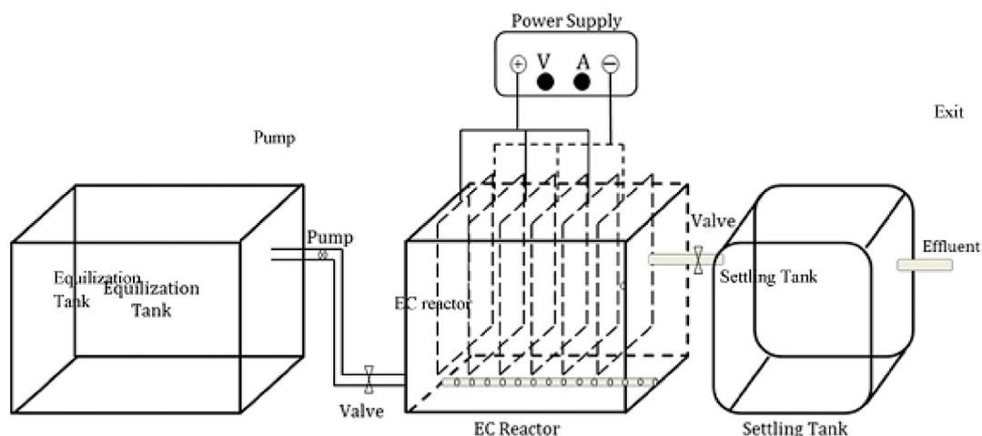
Figure 10. Schematic view of the pilot electrocoagulation plant [52].
