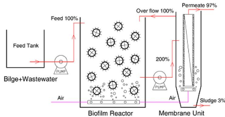
**Figure 13.** Recycle side-stream configuration of biofilm-MBR [67].
