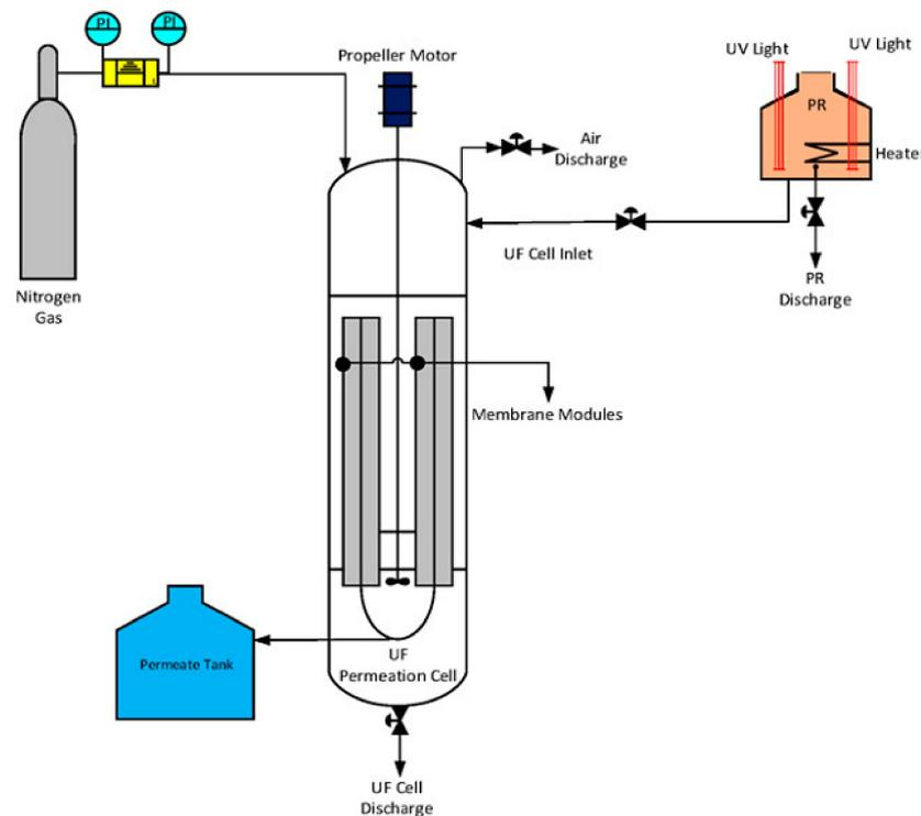
Figure 18. Schematic diagram of the PR-UF system [74].
