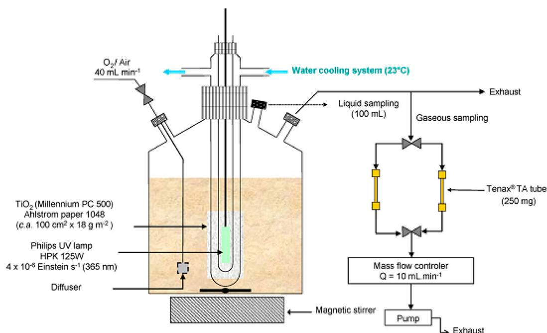
Figure 16. Schematic of the 1 L batch photo reactor [72].
