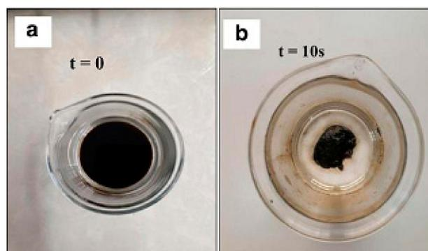
**Figure 5.** Digital photograph images of removal of crude oil from water surface by synthesized nanocomposite (a,b) [35].
