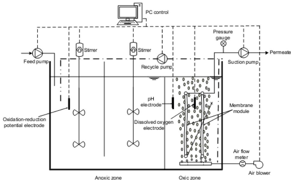
**Figure 14.** Schematic diagram of the pilot-scale A/O-MBR [68].
