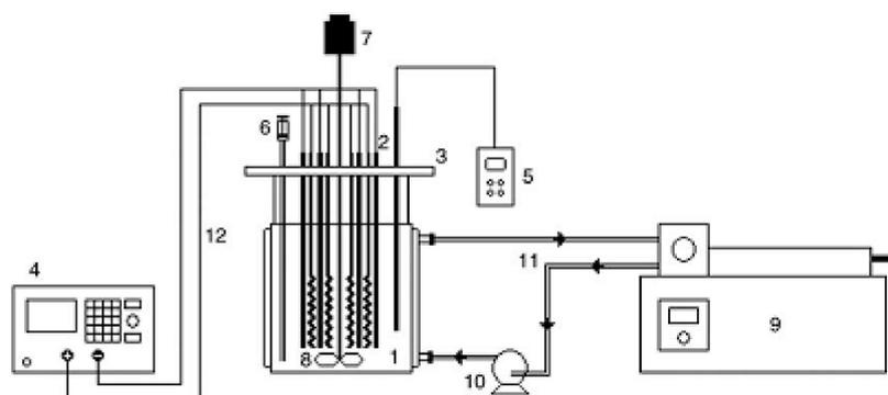
Figure 11. Batch electrochemical reactor system (1: stirred batch electrochemical reactor, 2: Pt/Ir anodes and Fe cathodes, 3: Polyamide@reactor lid, 4: programmable DC power source, 5: digital thermometer, 6: sampling cell, 7: driving motor, 8: glass mixer, 9: heating/cooling tank, 10: heating/cooling pump, 11: heating/cooling feed, 12: power supply connections) [53].
