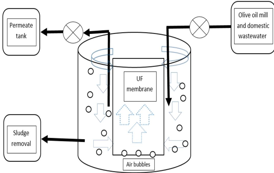
Figure S4. Schematic diagram of the MBR.
