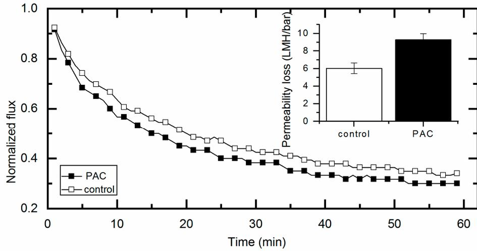
Figure S1. Flux decline during fouling with SMP ( $50 \pm 3$  mg/L TOC dissolved in DI water) and corresponding irreversible permeability loss after 60 minutes filtration of SMP solution originated from the two MBR with and without PAC.
