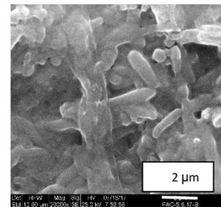
Figure S3. SEM images of the biofilm layers developed on membranes taken from the two MBR systems, with and without PAC.
