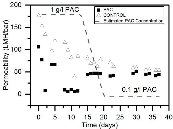
Figure S5. Permeability of the membranes in MBR-PAC and the control (w/o PAC) during the preliminary experiment. A rapid decline in the permeability of the membrane in the PAC reactor was observed versus slower decline in membrane permeability in the control reactor. Therefore, a gradual reduction in PAC concentration was performed. Once the PAC concentration in the reactor had reached the final concentration of 0.1 g/l, the permeability was close in the two reactors.
