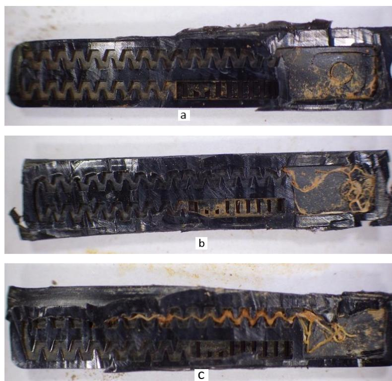
**Figure 12.** Photos of anatomical emitters: (a) no root intrusion; (b) roots that had entered into the water outlet of the emitter but had not entered into the channel; (c) roots that had entered into the emitter channel.
