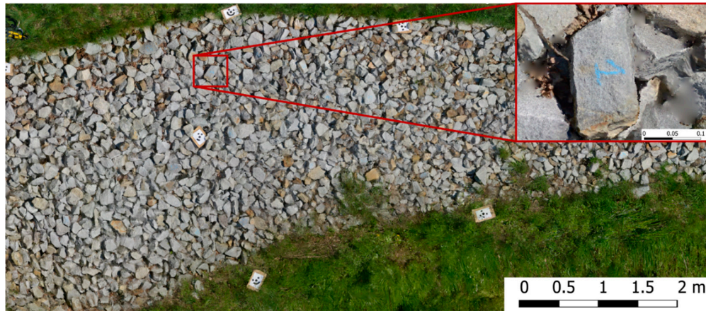
Figure 5. Validation dataset—orthomosaic created for the first epoch (before particle displacement). The white squares with black marks are the GCP targets. The enlargement shows one of the particles marked with a number. Marked particles were later displaced.
