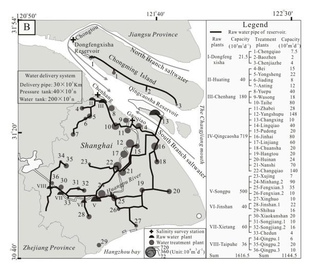
**Figure 1.** (**A**) Flow chart of the water supply system in Shanghai, (**B**) the distribution of raw water plants, water treatment plants and water delivery pipes in Shanghai in 2013, and the sites where water quality and threat factor data were collected.
