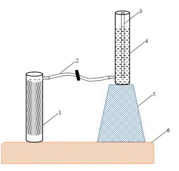
**Figure 1.** Experimental setup for one-dimension vertical water infiltration. (1) Soil column; (2) Water pipe; (3) Intake tube; (4) Markov bottle; (5) Retort stand; and (6) Desktop.
