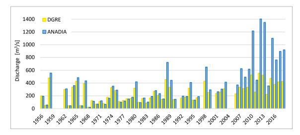
Figure 6. Comparison between the DGRE (yellow bars) and ANADIA (blue bars) time series of annual maximum discharge.
