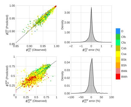
**Figure 4.** Performance evaluation of the random forests-based model (RFB) for the transition probabilities dry-dry and wet-wet for 1-h intervals. Results are shown in the same way as defined in Figure 3.
