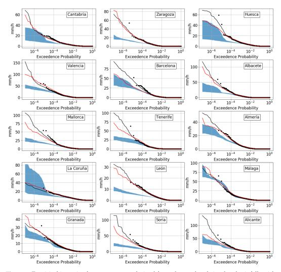
**Figure 8.** Empirical intensity-frequency curves derived from observed and simulated rainfall at 1-h aggregation. Black dots represent exceedance probability values of the observed rainfall series. Black and red lines correspond to the exceedance probability of "exact scenario" and "target scenario", respectively. The blue-colored area represents the range of exceedance probability values between the 10 calibrations in the "simple scenario". Each panel corresponds to a case study.
