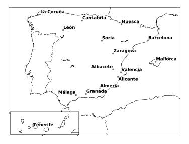
**Figure 5.** Location of the hourly rainfall gauges used to perform the simulation of the rainfall by the Neyman–Scott rectangular pulse model (NSRPM).
