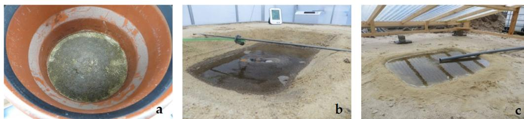
**Figure 2.** Infiltration basin: column (a), laboratory tank (b) and field infiltration unit (c).
