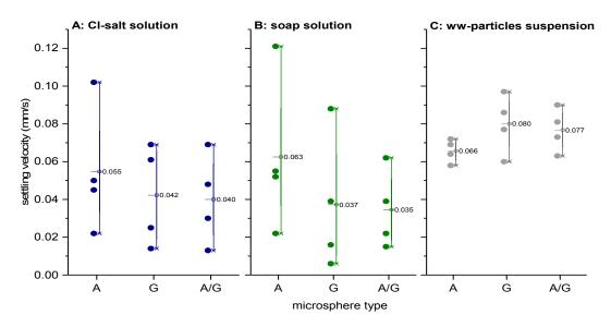
**Figure 3.** Settling velocity of microspheres with different surface coatings (protein A, G and A/G) in Cl-salt solution (**A**), soap solution (**B**) and wastewater particles suspension (**C**).
