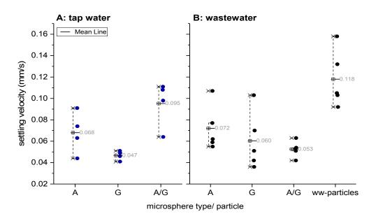
**Figure 2.** Settling velocity of microspheres with different surface coatings (protein A, G and A/G) in tap water (**A**) and wastewater (ww) (**B**).
