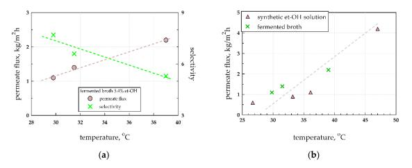
**Figure 7.** (a) Permeate flux and selectivity versus the feed solution temperature for fermented broth solutions; average ethanol concentration 5.4% v/v; and (b) comparison of synthetic ethanol solutions and fermented broth solutions.
