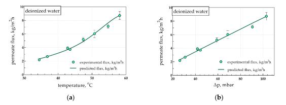
**Figure 9.** Comparison between values predicted by the model and experimental vapor flux data. Permeate flux versus: (a) the feed solution temperature, and (b) the driving force (vapor pressure-applied vacuum). Data from deionized water distillation.
