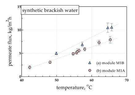
**Figure 5.** Permeate flux versus the feed solution temperature for the desalination of synthetic brackish water. Effective membrane area (**a**) module M1B, 0.067 m<sup>2</sup>, and (**b**) module M1A, 0.087 m<sup>2</sup>.
