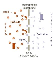
Figure 1. Membrane distillation (MD) principle.
