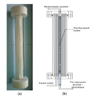
**Figure 2.** (a) A view of M1 custom-made vacuum membrane distillation (VMD) module; (b) a cross-sectional view of M2 VMD module.
