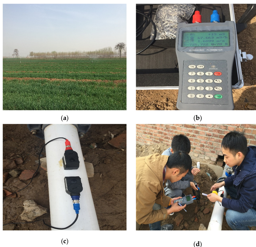
Figure 3. Pumping test in the field. (a) Wheat field in project region; (b) Handheld Ultrasonic Flow Meter (Flowmeter, HT-003UF, Beijing, China); (c) The sensor of Handheld Ultrasonic Flow Meter (Flowmeter, HT-003UF, Beijing, China); and (d) Experimental field. The photos were taken by Dr. Xu Ting in the project region in Houcun, Quzhou County on 30 March 2016; there are no copyright issues for these pictures.
