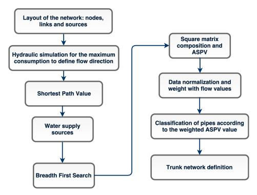
Figure 1. Flowchart to obtain the Trunk Network.
