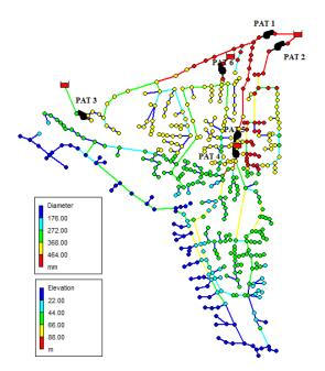
Figure 12. Balerma Irrigation network and PATs location.
