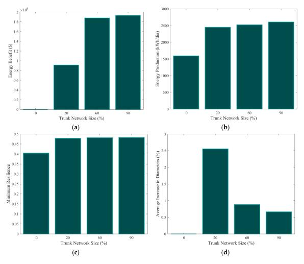
**Figure 14.** Results of TN rehabilitation for the Balerma irrigation network: (**a**) Energy benefit; (**b**) Energy produced; (**c**) Minimum resilience; and, (**d**) Average increase in pipes diameters.
