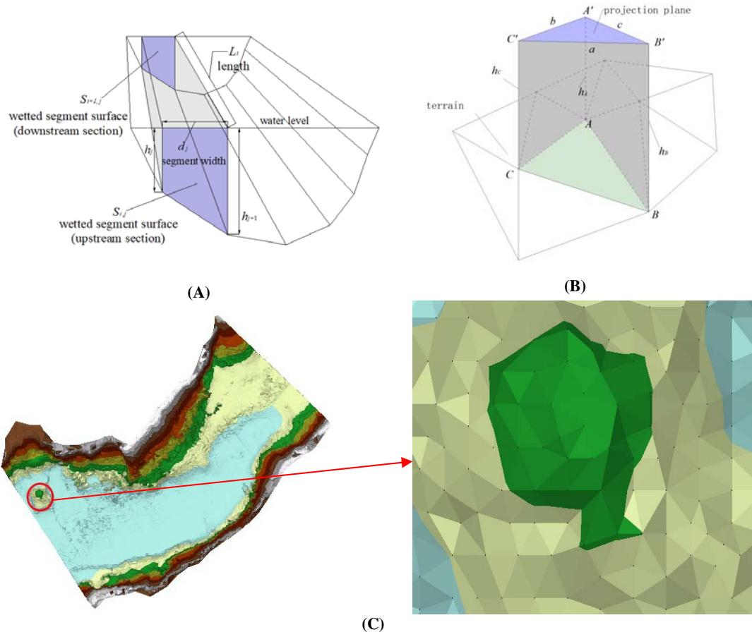
**Figure S3.** The storage capacity calculation method. **(A)** Cross-section Method; **(B)** Triangle Prism Method; and **(C)** Triangulated Terrain between M13 and M14.
