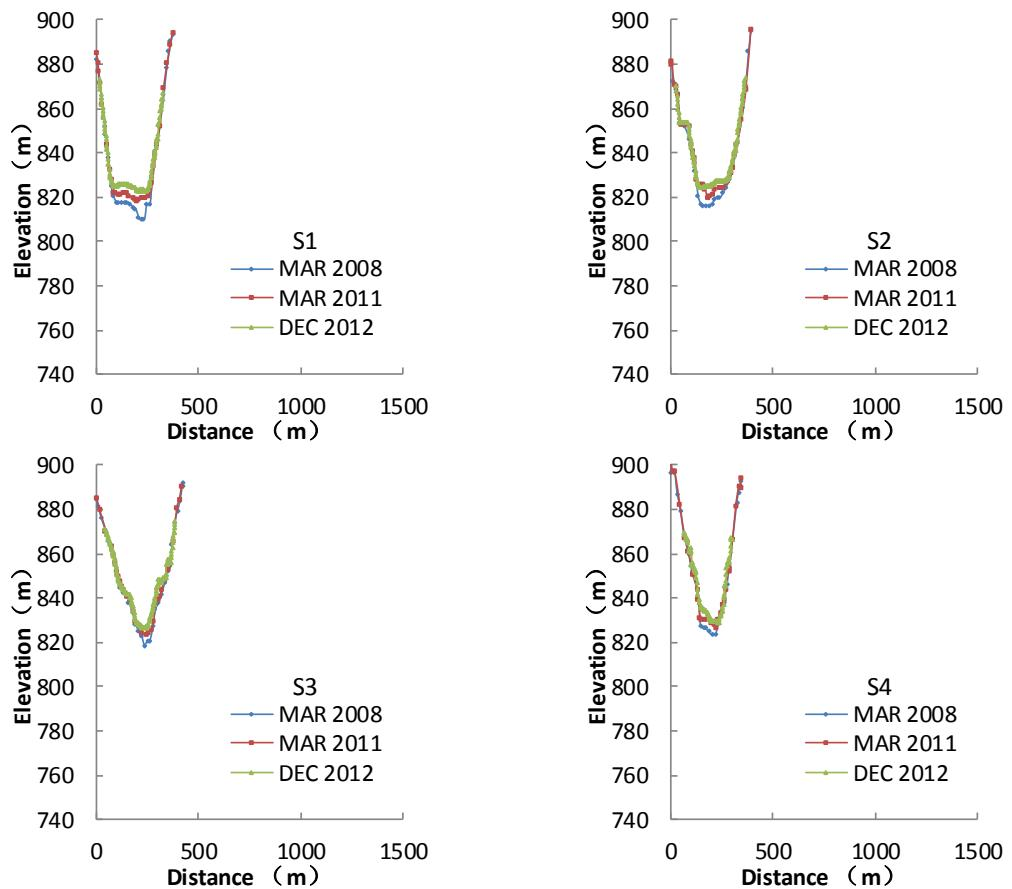
**Figure S4.** The topographic profiles of all cross sections
