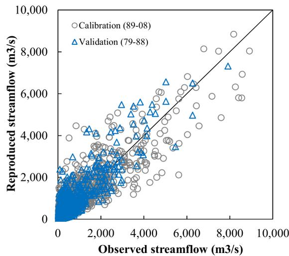
**Figure 5.** Scattered plot of daily observed and reproduced streamflow for the upper Thu Bon River basin at Nong Son in the calibration period (1989–2008) and validation period (1979–1988).
