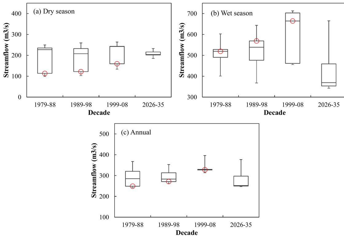
**Figure 11.** Box-and-whisker plot of (a) dry season, (b) wet season, and (c) annual streamflow simulated using high-resolution multi-model simulations for each decade in the baseline and near-term climates; the red circles represent mean streamflow simulated using observed rainfall.
