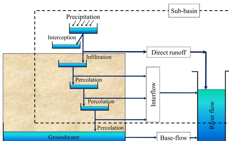
**Figure 1.** Schematic of the super-tank model, modified after [19].
