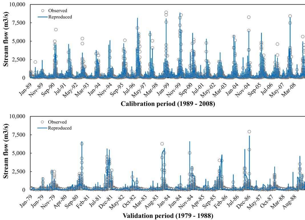
**Figure 4.** Time series of the daily observed and reproduced streamflow for the upper Thu Bon River basin at Nong Son: (**Upper**) calibration period (1989–2008) and (**Lower**) validation period (1979–1988).
