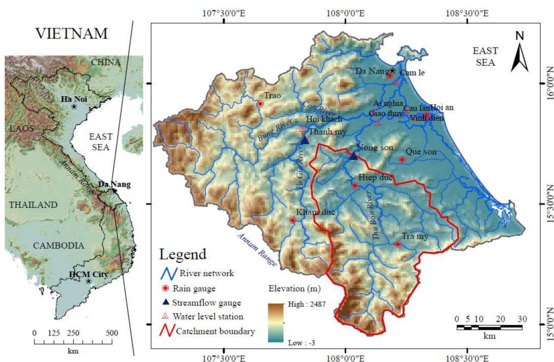
**Figure 2.** Map of the upper Thu Bon River basin as delineated at Nong Son stream gauge and locations of hydro-meteorological observation, modified after [11].
