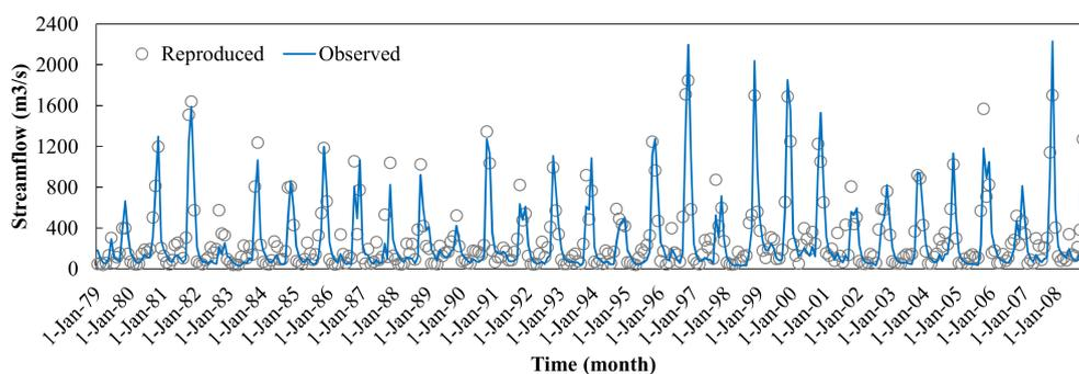
**Figure 6.** Time series of monthly observed and reproduced streamflow for the upper Thu Bon River basin at Nong Son in the period of 1979–2008.
