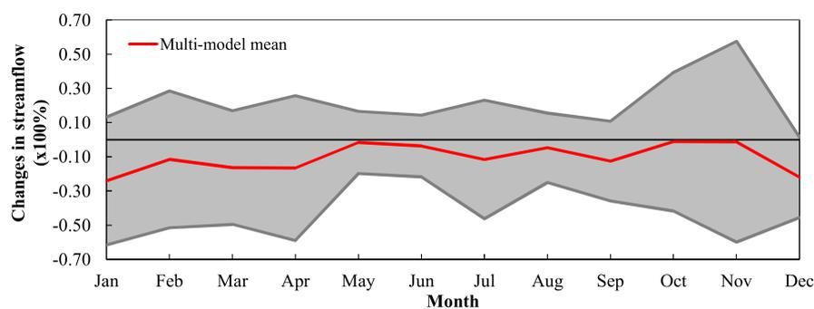
**Figure 10.** The 95 percent confidence interval of changes in the average monthly streamflow in the near-term (2026–2035) climate simulated using projected rainfall, relative to the baseline (1979–2003) climate.
