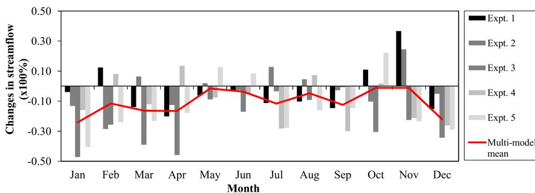
**Figure 9.** Changes in average monthly streamflow in the near-term (2026–2035) climate simulated using projected rainfall, relative to the baseline (1979–2008) climate.
