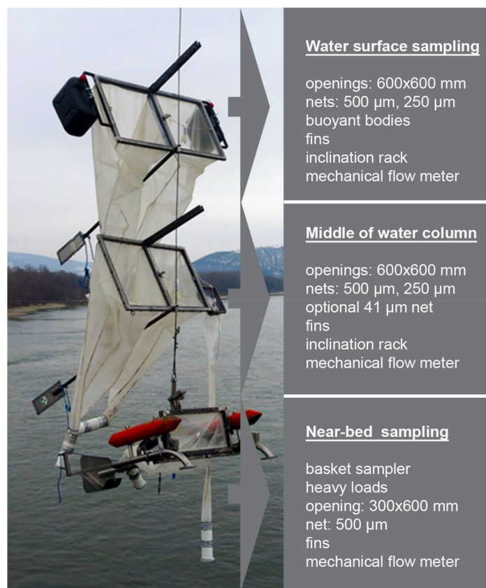
Figure 2. Final device configuration used for collecting measurements in the Austrian Danube River.
