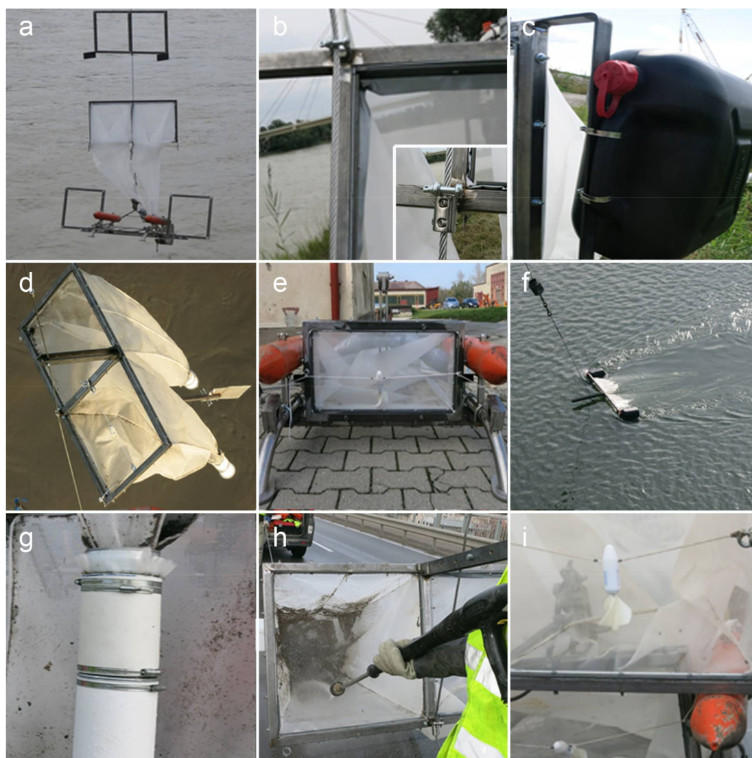
Figure 1. Pictures depicting the development of the device: (a) first prototype with small fins and 600 \times 600 \text{ mm} frames at each level; (b) steel rope and shackles, and adjustable stopper to keep the net assemblage at the right position; (c) buoyant body to ensure near-surface skimming; (d) long fin and inclination rack for good positioning; (e) centred single net near the bed; (f) upright position when inside the water; (g) sampling container to reduce the emptying time; (h) high-pressure cleaning of the nets; (i) mechanical flow meter to measure the discharge through the nets.
