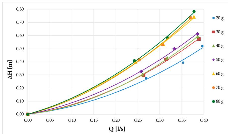
**Figure 9.** Results of all tests of clogging with fine sand in terms of head losses as functions of discharges for the three different discharges.
