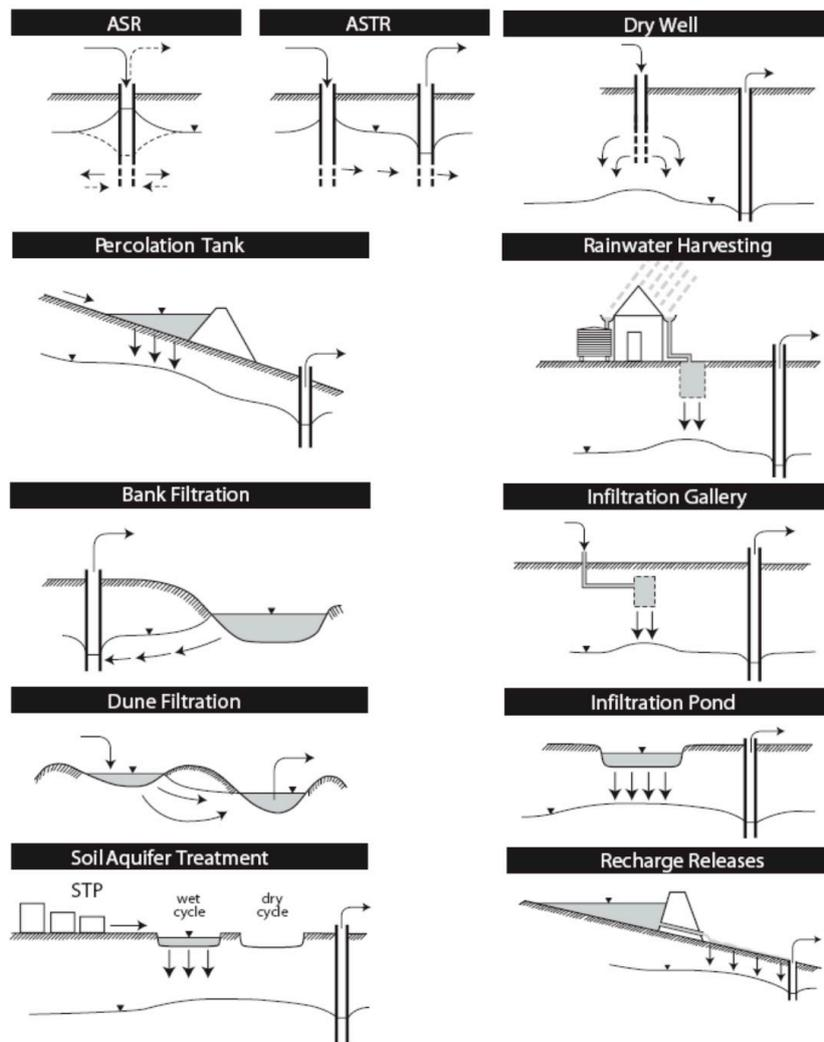
**Figure 1.** Schematic of types of MAR suited to urban water management (modified from: Dillon, 2005 [2]). ASR—Aquifer Storage and Recovery; ASTR—Aquifer Storage Transfer Recovery; STP—Sewerage Treatment Plant.
