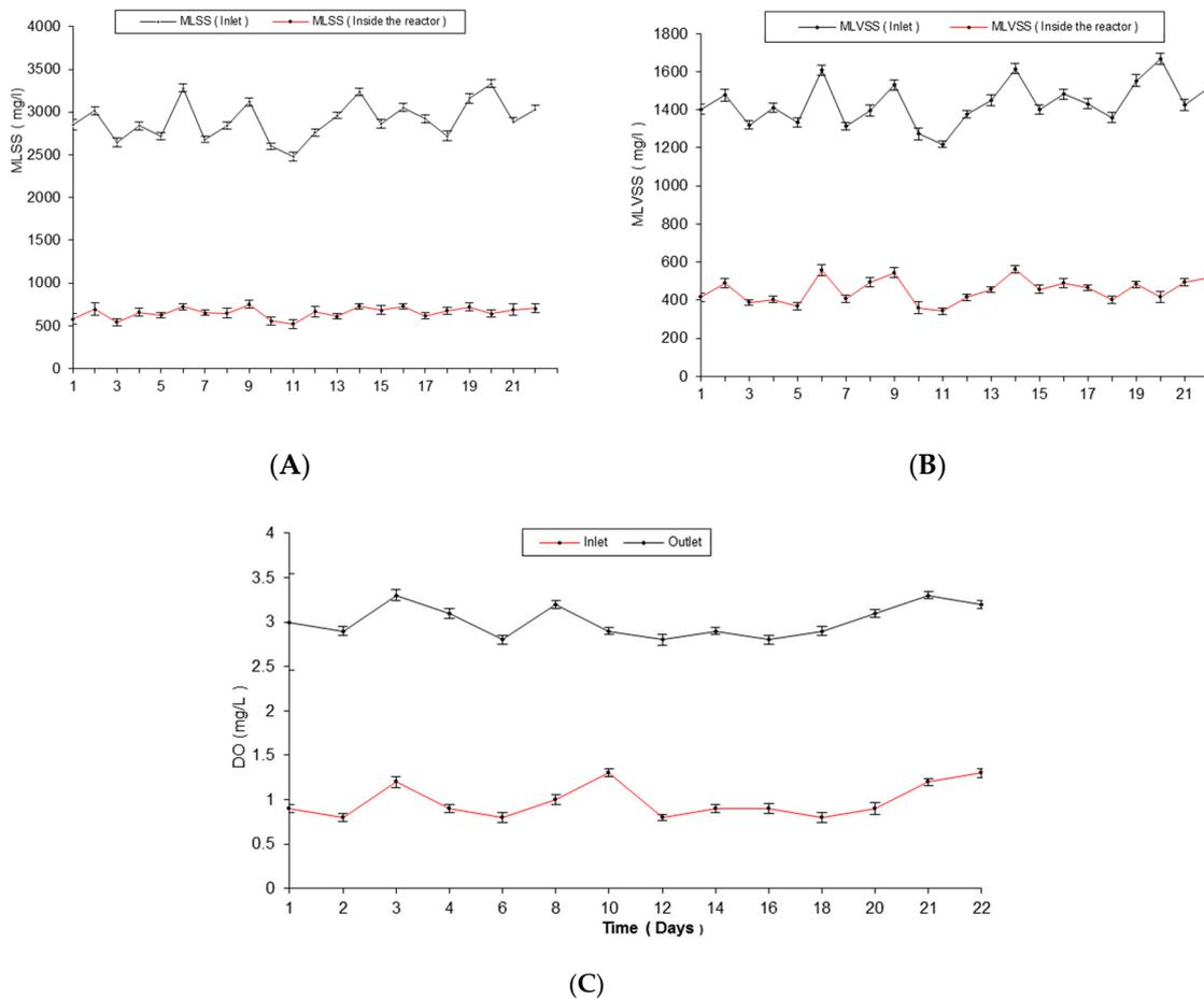
**Figure 4.** (A) MLSS profile in continuous mode aerobic digester (MBBR sludge); (B) MLVSS profile in continuous mode aerobic digester (MBBR sludge); (C) DO profile in continuous mode aerobic digester (MBBR sludge).
