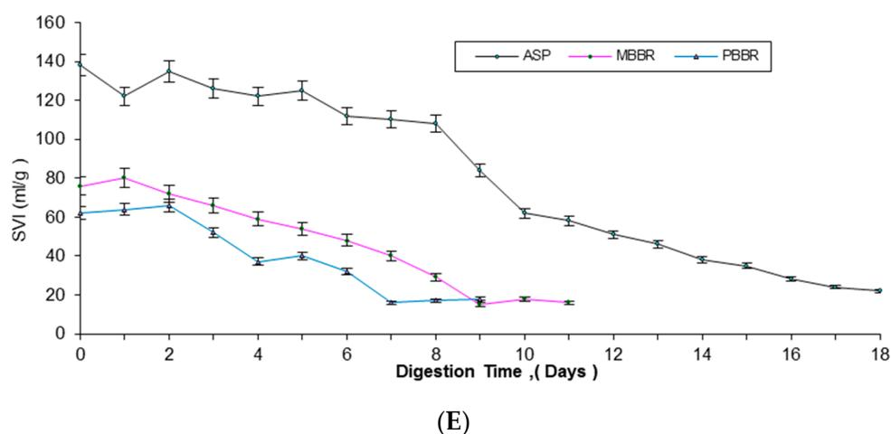
**Figure 2.** Variation in \* MLSS (A), MLVSS (B), COD (C), and DO (D) SVI (E) during batch aerobic digestion. \* legend MLSS: Mixed Liquor Suspended Solid; MLVSS: Mixed Liquor Suspended Solid; COD: Chemical Oxygen Demand; DO: Dissolved Solid; SVI: Sludge Volume Index.
