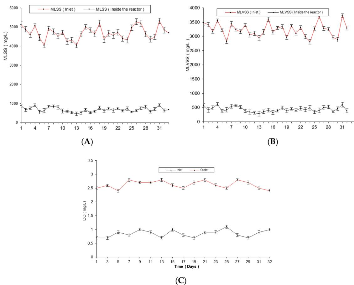
**Figure 3.** (A) MLSS profile in continuous mode aerobic digester (ASP sludge); (B) MLVSS profile in continuous mode aerobic digester (ASP sludge); (C) DO profile in continuous mode aerobic digester (ASP sludge).
