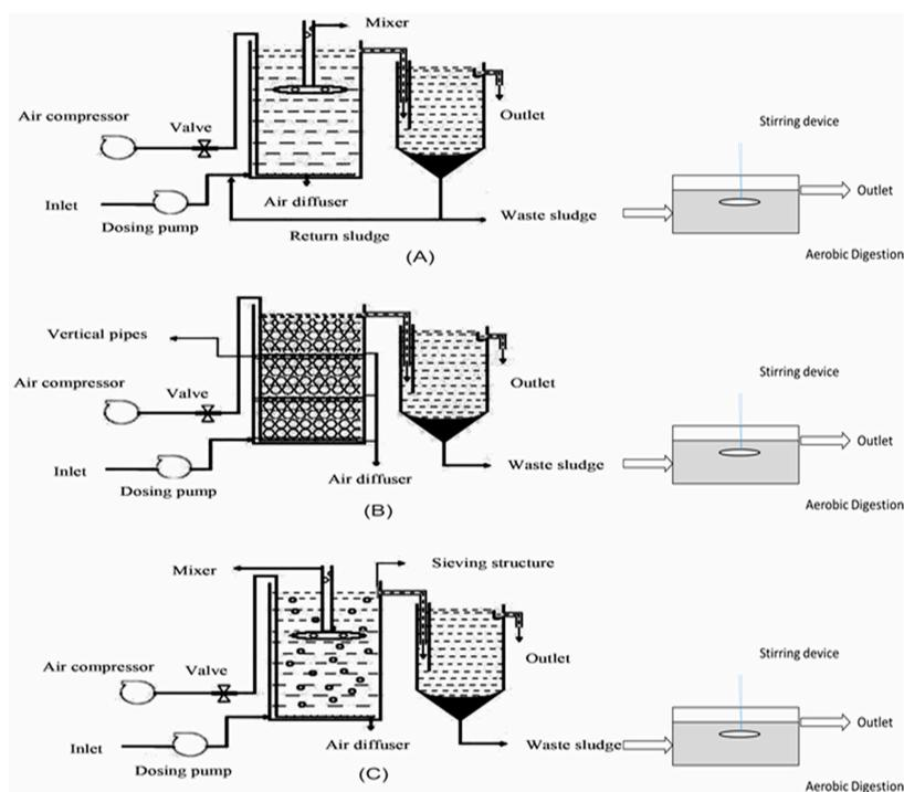
**Figure 1.** The schematic appearance of biological treatment process in the presence of an aerobic digester (A) ASP: Activated Sludge Process, (B) PBBR: Packed Bed Biofilm, (C) MBBR: Moving Bed Bioreactor.
