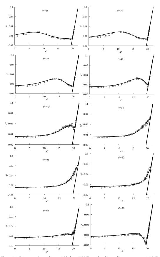
**Figure 3.** Run-up and run-down of  $H_w/h_0 = 0.0185$  non-breaking solitary wave on a 1:19.85 sloping beach.
