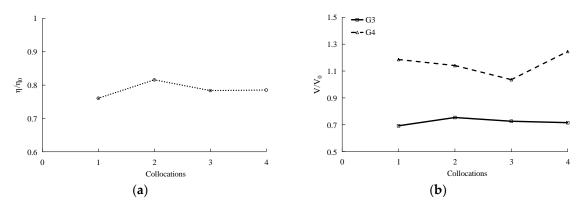
**Figure 17.** Variation of normalized run-up heights and normalized peak flow velocities at G3 and G4 with different tree collocations, (**a**) The normalized run-up heights, (**b**) The normalized peak flow velocities.
