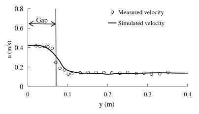
**Figure 8.** Transverse profiles of maximum velocity in a cross-section of Gage 6 ( $B_g = 0.07$  m).
