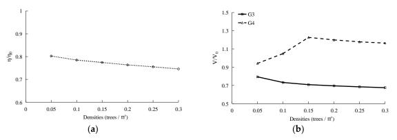
**Figure 18.** Variation of normalized run-up heights and normalized peak flow velocities at G3 and G4 with different densities of pure *P. odoratissimus*. (**a**) The normalized run-up heights, (**b**) The normalized peak flow velocities.
