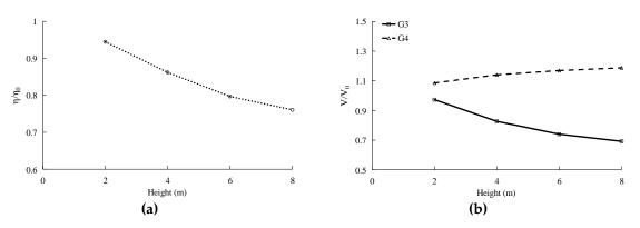
**Figure 19.** Variation of normalized run-up heights and normalized peak flow velocities at G3 and G4 with different heights of pure *P. odoratissimus*; (**a**) The normalized run-up heights, (**b**) The normalized peak flow velocities.
