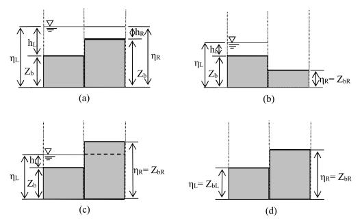
Figure 1. Schematic diagram of wet-dry edges.
