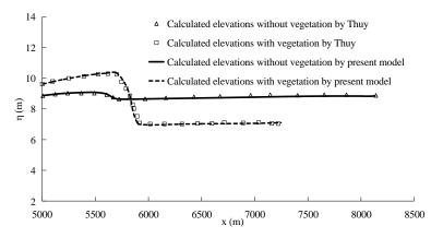
**Figure 10.** Maximum water surface elevations of the first wave without vegetation and with *P. odoratissimus* vegetation [26].
