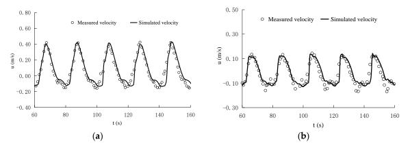
**Figure 7.** Time series of velocities, (**a**) at the center of the gap exit, (**b**) at the center of the end of the vegetation.
