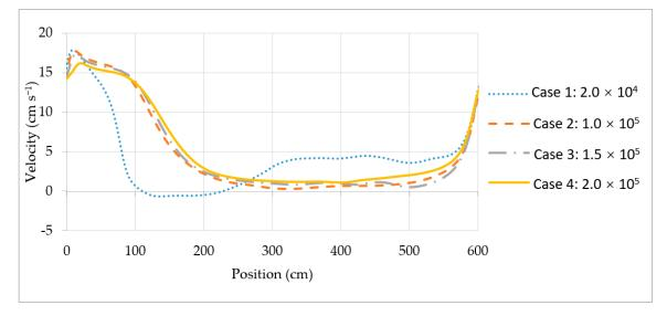
Figure 1. Grid convergence for different cell sizes.
