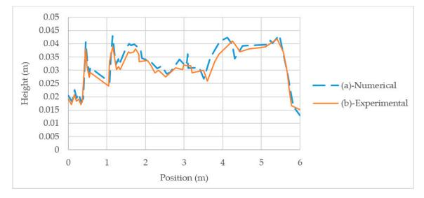
Figure 3. Profile of deposition in the reservoir for (a) numerical and (b) experimental data [35].
