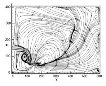
Figure 6. Stream Lines 15.5 cm from the bed, G374 reservoir.
