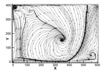
Figure 8. Stream Lines 15.5 cm from the bed, G3716 reservoir.
