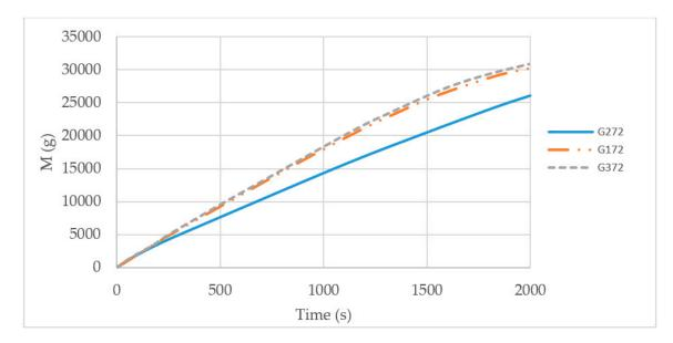
Figure 4. Amount of deposition in the three reservoirs over 2000 s.
