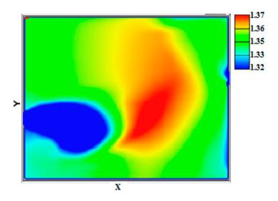
Figure 5. The pattern of sediment deposition in G374 reservoir.
