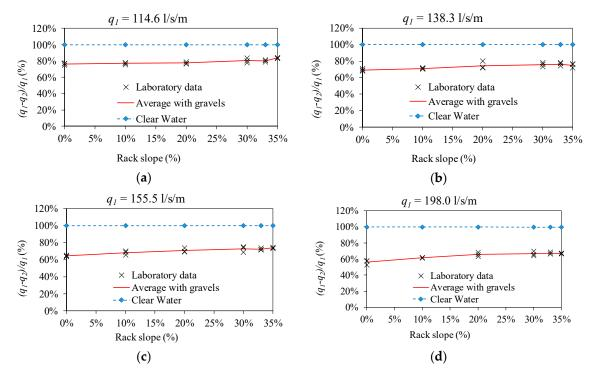
**Figure 6.** Percentage of derived flow for a specific inlet flow: **(a)** 114.6 l/s/m; **(b)** 138.3 l/s/m; **(c)** 155.5 l/s/m; **(d)** 198.0 l/s/m.
