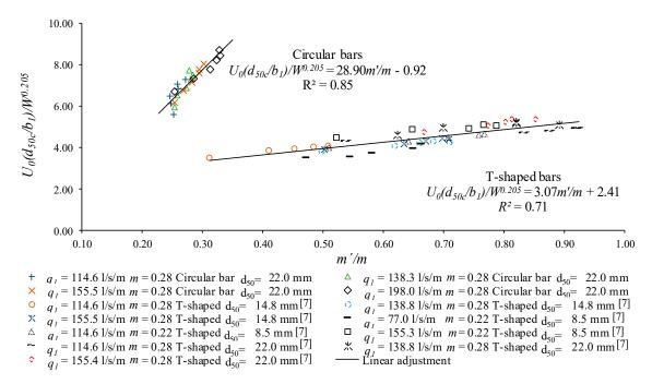
**Figure 19.** Linear adjustment of the ratio m'/m ratio as a function of the values  $U_0$ ,  $d_{50c}/b_1$ , and W.
