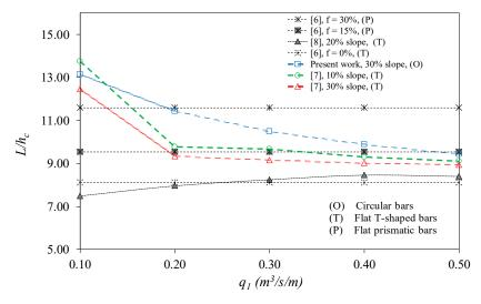
**Figure 20.** Calculated rack length necessary to derive the total incoming flow when sediment transport is presented for different rack slopes.
