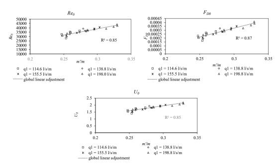
**Figure 14.** Velocity at the beginning of the rack,  $U_0$ , as a function of the ratio between the effective and the initial void ratios, m'/m.
