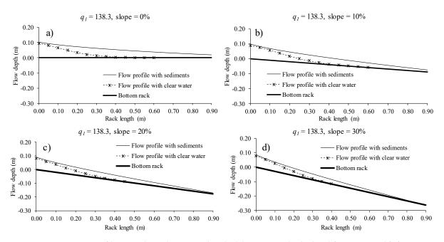
**Figure 11.** Water profiles over the rack measured in the laboratory and calculated for  $q_1 = 138.3 \text{ l/s/m}$  and slopes (a) 0%; (b) 10%; (c) 20%; and (d) 30%.
