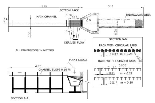
Figure 4. Scheme of the intake system physical device.
