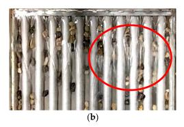
**Figure 9.** Flow over the occluded circular bars bottom rack and formation of wakes for rack slopes: (a) 20%; (b) 30%.
