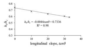
**Figure 15.** Ratio  $h_0/h_c$ , which is dependent on the rack slope, according to Reference [23].
