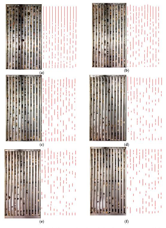
**Figure 7.** Top view of occluded bottom racks with circular bars for m = 0.28,  $q_1 = 138.3 \text{ l/s/m}$ , and diverse longitudinal slopes: (a) 0%; (b) 10%; (c) 20%; (d) 30%; (e) 33%; and (f) 35%.
