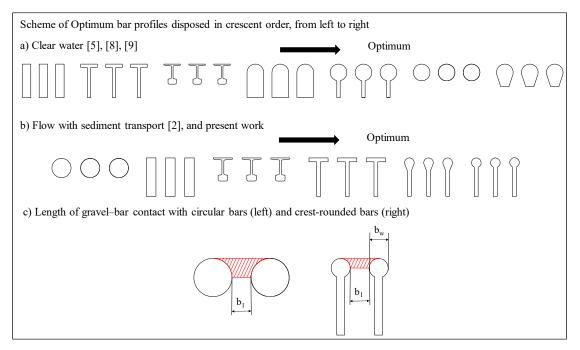
**Figure 3.** Scheme of optimum bar profiles: (a) clear water flow; (b) flow with sediments; (c) comprehensive sketch to visualize the influence of the profile radius on the length of gravel–bar contact.
