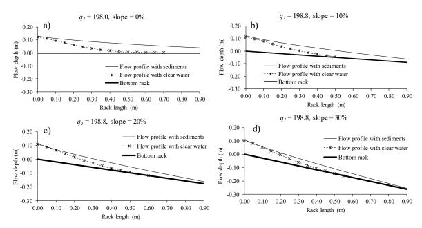
**Figure 13.** Water profiles over the rack measured in the laboratory and calculated for  $q_1 = 198.0 \text{ l/s/m}$  and slopes (a) 0%; (b) 10%; (c) 20%; and (d) 30%.
