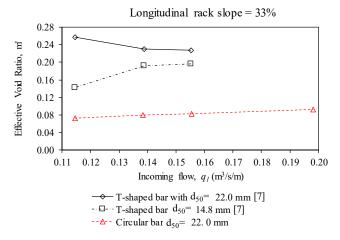
**Figure 17.** Comparison of effective void ratio, m', for circular bars and values previously presented for T-shaped bars [7]. All cases have a void ratio of m = 0.28.
