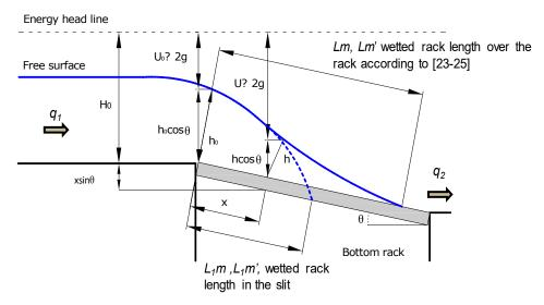
Figure 5. Scheme of the spatially varied flow over the bottom intake system.
