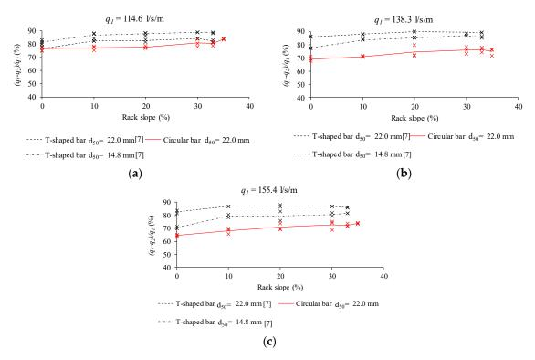
**Figure 16.** Comparison between percentage of derived flow for bottom racks with T-shaped bars (gravel 2 and gravel 3) and circular bars (gravel 3) for specific inlet flows: (a) 114.6 l/s/m; (b) 138.3 l/s/m; and (c) 155.5 l/s/m.
