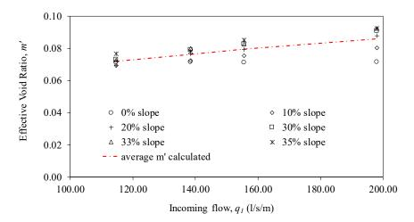
**Figure 10.** Effective void ratio values, m', for different rack slopes and incoming flows.
