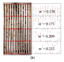
**Figure 8.** Top view of occluded bottom racks with circular bars for m = 0.60, dividing the rack into four parts, with the void ratio calculated from occluded areas: (a)  $q_1 = 155.5 \text{ l/s/m}$  and 10% longitudinal slope and (b)  $q_1 = 198.0 \text{ l/s/m}$  and 35% longitudinal slope.
