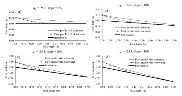
**Figure 12.** Water profiles over the rack measured in the laboratory and calculated for  $q_1 = 155.5 \text{ l/s/m}$  and slopes (a) 0%; (b) 10%; (c) 20%; and (d) 30%.
