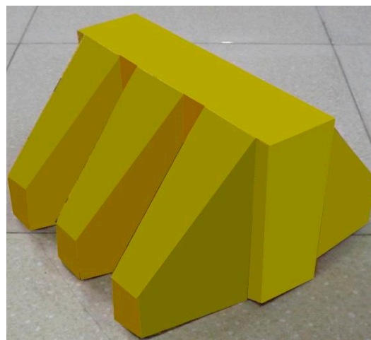
Figure 7. A single block model of a spur dike with tooth-shaped structures.
