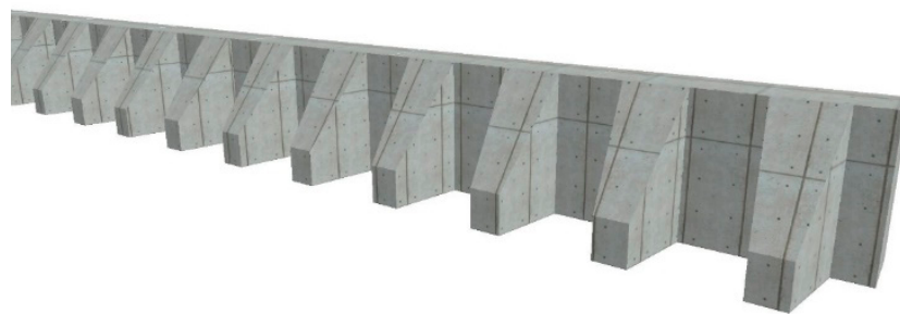
Figure 6. A row of a spur dike with tooth-shaped structures.
