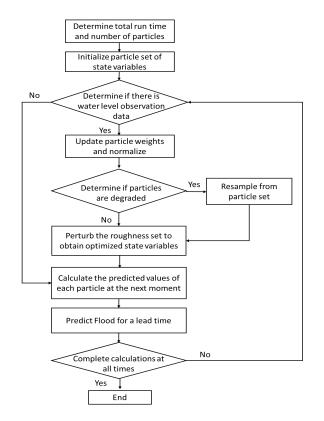
Figure 2. Flow chart of the hydrodynamic assimilation system.
