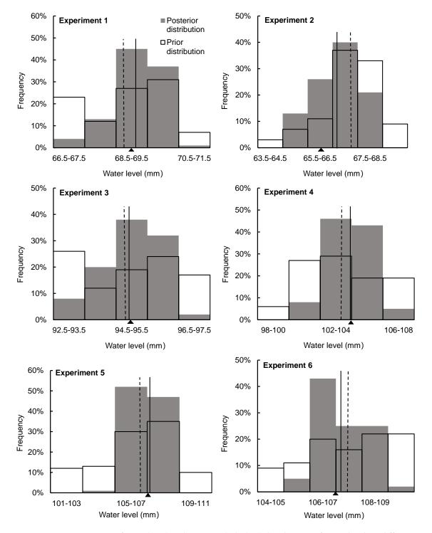
**Figure 5.** Histograms of prior (gray) and posterior (colorless) distributions of water levels in different experiments. The observed value is marked with a black triangle. The black dotted line indicates the mean value of the prior distribution of particles and the black solid line indicates the mean value of the posterior distribution of particles.
