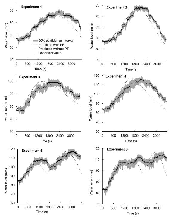
**Figure 4.** Comparison between observed and predicted water level processes. The dots represent the observed values. The black line represents the mean of the particles simulated by assimilation model. The dotted line represents the water level calculated by the hydrodynamic model. The gray shaded area represents the 90% confidence interval.
