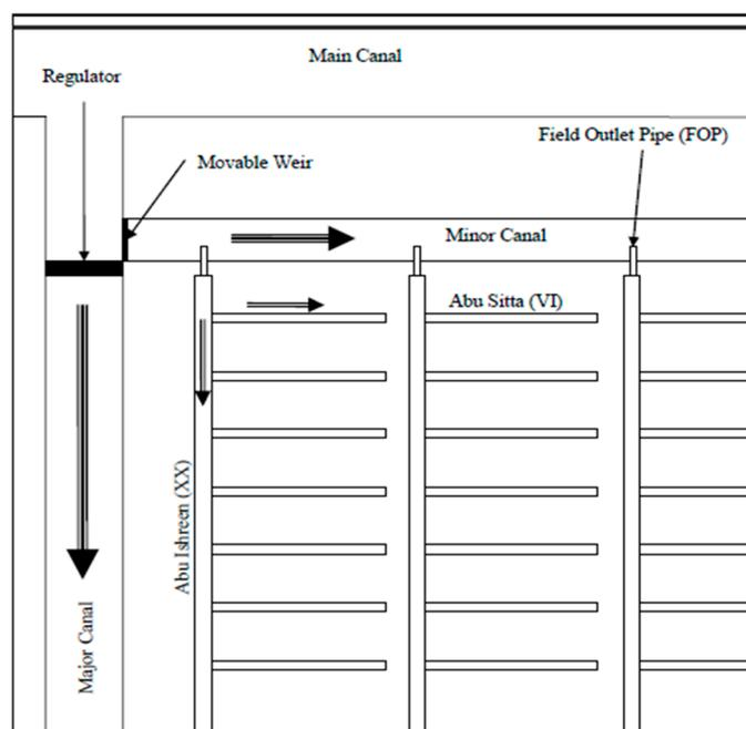
**Figure 2.** Field irrigation system in Gezira scheme.
