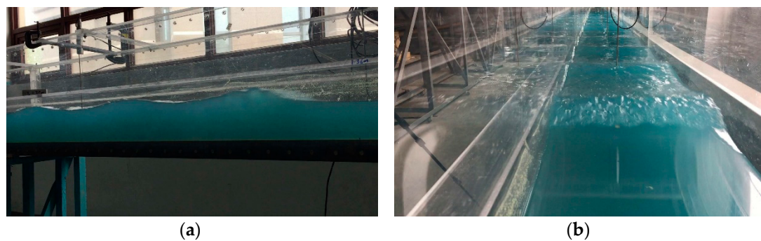
Figure 3. Breaking undular surges in Stage 3: (a) Lateral view; (b) looking upstream at the incoming wave.
