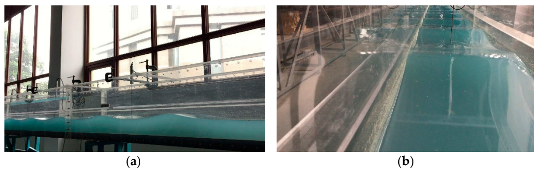
Figure 2. Non-breaking undular surges in Stage 2b: (a) Lateral view; (b) looking upstream at the incoming wave.
