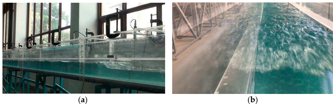
Figure 4. Breaking surges in Stage 4: (a) Lateral view; (b) looking upstream at the incoming wave.
