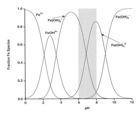
Figure S1. Fe(III) speciation as a function of water pH
