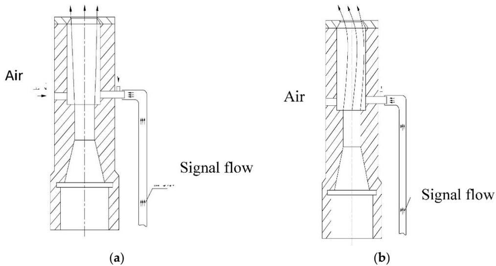
**Figure 2.** (a) Straight main flow jet. (b) Main flow jet reattached to the right.
