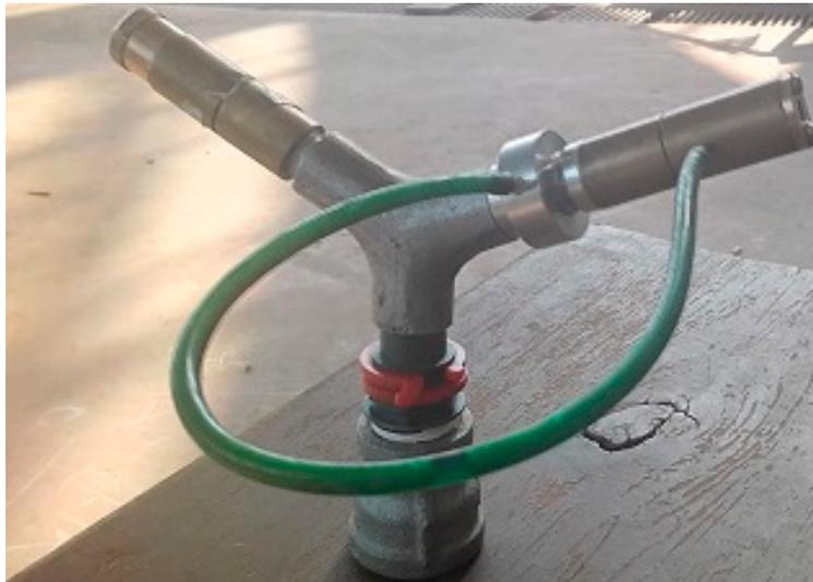
**Figure 3.** Prototype of the dynamic fluidic sprinkler.
