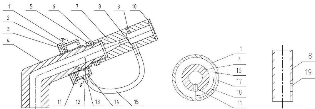
**Figure 1.** Schematic, pictorial view of the new fluidic sprinkler head. 1. Water signal tank. 2. First lock nut. 3. Pipe sprayer. 4. Spray body. 5. Second lock nut. 6. Body of the fluidic element. 7. Jet element body. 8. Water inlet. 9. First air hole. 10. Outlet cover plate. 11. Water dividing hole. 12.  $\alpha$  main flow. 13. Signal nozzle. 14. Third lock nut. 15. Conduit. 16. Water storage capacity. 17. Signal hole. 18.  $\beta$  contraction angle. 19. Second air hole.
