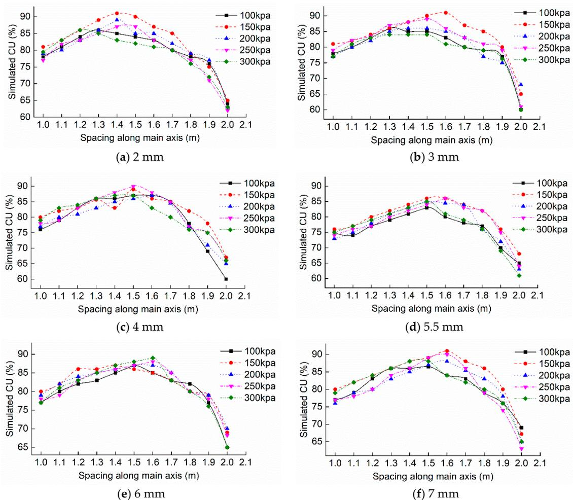
**Figure 6.** Computed coefficient of uniformity (CU) for different types of nozzles and pressures.
