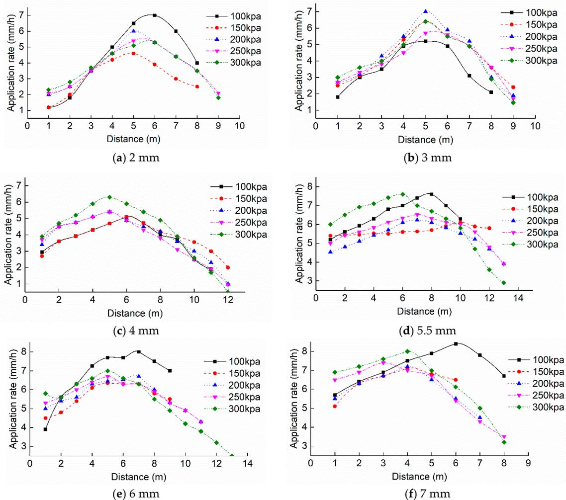
Figure 5. Water distribution profiles for different types of nozzles and pressures.
