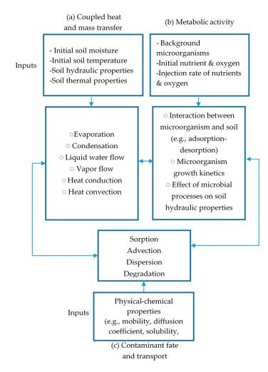
**Figure 2.** Mathematical modeling framework for a fully coupled thermally enhanced bioremediation– energy storage system.
