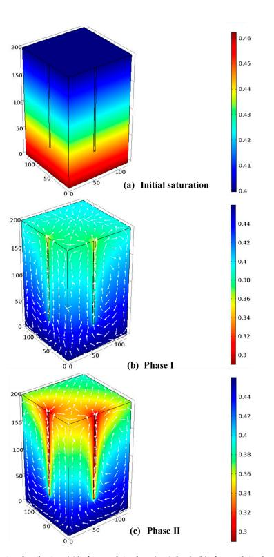
**Figure 5.** Saturation distribution: (**a**) before applying heat (t = 0 days); (**b**) after applying heat in phase I (t = 4 days) and (**c**) after applying heat in phase (II) (t = 4 days). Arrows in figure (**b**,**c**) show the gas phase velocity field.
