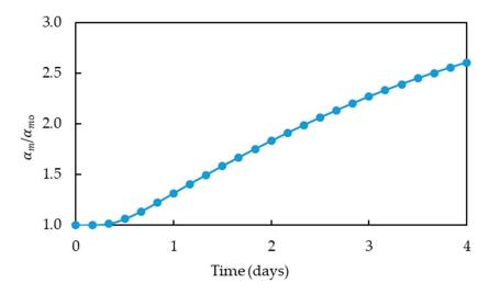
**Figure 6.** Ratio of carbon dioxide production after applying heat with respect to the reference value of carbon production at initial temperature ( $\alpha_m / \alpha_{mo}$ ) at a single point located in the middle of the domain.
