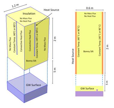
**Figure 3.** Three- and two-dimensional schematics of the simulated domain as well as boundary conditions used in the simulation. Due to symmetry, only a quarter of the domain is modeled. The line heat sources have a constant temperature (40 °C or 80 °C). The side boundaries are modeled as convective heat transfer boundaries. It is assumed that the surface of the domain is insulated (GW: Ground Water).
