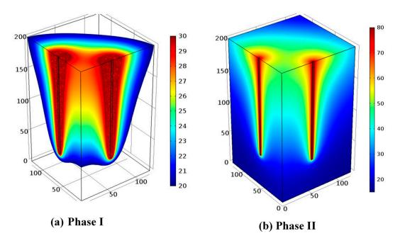
**Figure 4.** Temperature (°C) distribution in the domain after 4 days for (**a**) remediation phase and (**b**) storage phase. For the remediation phase, the part of the domain that has a temperature between 20-30 °C is shown. Only a quarter of the domain is presented.
